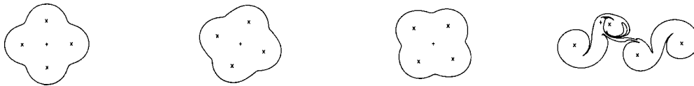
FIG. 18. Nonlinear response of a pentapolar vortex ( a=1.65 ) to a perturbation in which all satellite line vortices are moved outwards by 0.1. This structure is linearly unstable with a linear growth rate of approximately 0.1. The structure rotates steadily for a while but by t=7.5 (roughly the e -fold time according to linear theory) it has eventually disintegrated. Times shown are t=0, 2.5, 5, and 7.5 .
