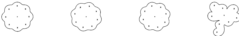
FIG. 20. Nonlinear response of an 8-polar vortex with a=1.4 to a perturbation in which all satellite line vortices are moved outwards by 0.1. This configuration has a maximum linear growth rate of 0.31. Times shown are t=0, 2.5, 5, and 7.5 . The configuration rotates steadily for a while, but by t=7.5 (roughly the e -fold time according to linear theory) the structure has disintegrated.
