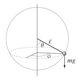
Figure 1: Spherical pendulum:  $x = R \sin \theta \cos \phi$ ,  $y = R \sin \theta \sin \theta$ ,  $z = -R \cos \theta$ .
