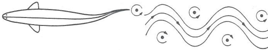
FIG. 11. Illustrating vortices cast off by the caudal-fin trailing edge as the fish moves to the left, and also the jet-like streamline pattern induced by those vortices (Lighthill 1969, after Karman & Burgers 1934).
