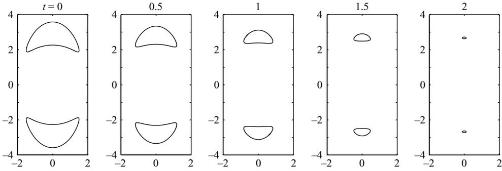
FIGURE 4. The evolution given by the exact solution driven purely by surface tension with  $\beta = 0$ . The bubbles shrink to zero area at a point.
