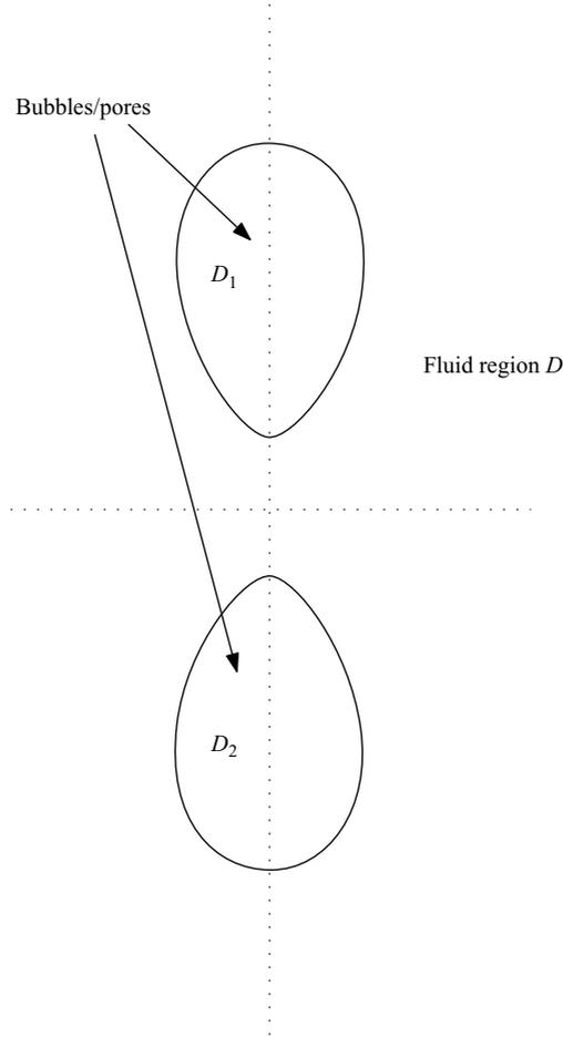
FIGURE 1. Schematic illustrating the flow configuration. The fluid region  $D$  is exterior to two bubbles (or ‘pores’)  $D_1$  and  $D_2$ . The two bubbles are reflectionally symmetric about both the  $x$ - and  $y$ -axes.
