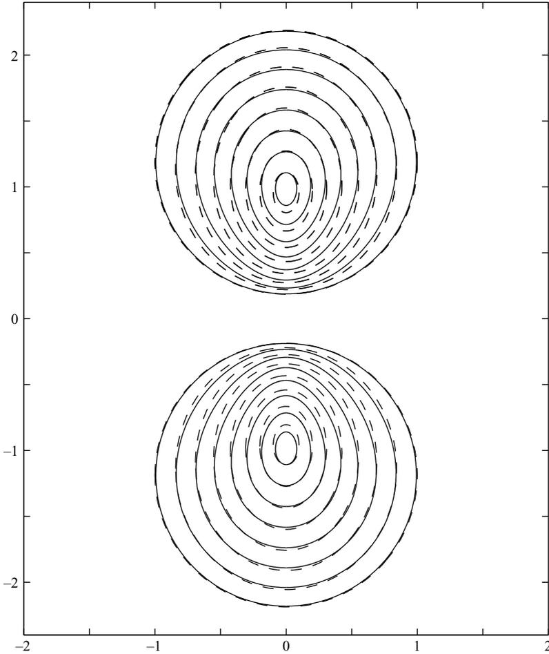
FIGURE 6. Comparison of the numerical simulation of pore closure with the elliptical pore model. The figure shows pore closure driven purely by surface tension with  $\rho(0) = 0.3$ ,  $\beta = 0$ . The solid lines are the results given by the full numerical simulation, the dashed lines are the results given by the elliptical pore model. Times shown are  $t = 0, (0.25), 1.75$ .
